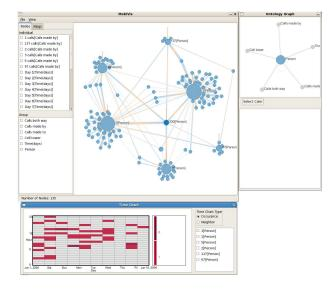
Figure 1: Overview of MobiVis. The central view provides a forcedirected layout of cell phones, where a link indicates communication between them. The upper right corner shows the ontology graph, which allows the user to highlight entity types of interest, such as people, calls and cell towers. The bottom view shows the interactive time chart, where color boxes denote time periods of activity.
