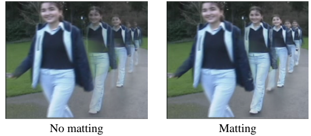
Figure 6: Alpha matting can be used to improve the blending of foreground objects. Left: no matting results in bleeding of background pixels to the other replicas. Right: matting results in crisper foreground objects (Video courtesy of Dan B Goldman).
