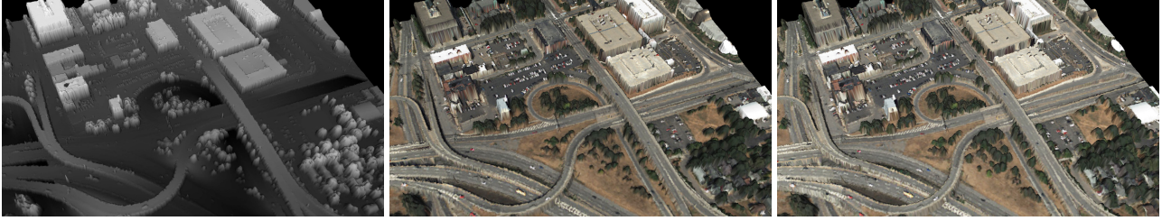
Figure 3. Registration results. From left to right , the untextured 3D LiDAR model (height map), a manually registered 3D model, and a 3D model generated by our registration process. Lighting and shading added, as in Figure 2.
